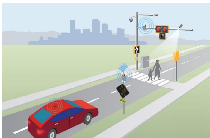
Figure 4. Example of Pedestrian Detection and Advanced Warning
